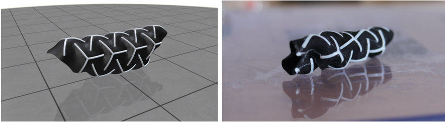
Figure 3: Our simulation tool (left) correctly predicts that a uniform star pattern, with free boundary, rolls up into a cylinder at static equilibrium (right). This complex behavior is due to the extrinsic curvature induced by the bilayer structure of the rod-and-fabric assembly, and the coupling of the bending of neighboring stars causing global symmetry-breaking in the pattern.
